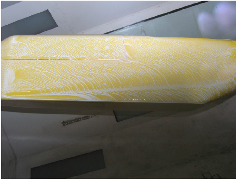
Fig. 21. Model B: flow visualization on port side for pitch = 20° and roll = 20°; flow from left to right.
