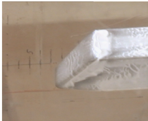
Fig. 8. Model A: flow separation at the nose–body junction next to leeside edge (pitch = 20^\circ , roll = 0^\circ ); flow from left to right.
