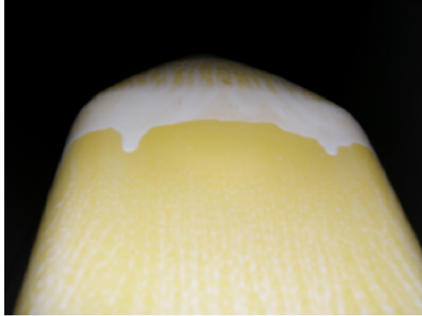
Fig. 18. Model B: separation bubble at the nose–afterbody junction leeward (pitch = 20°, roll = 0°, yaw = 0°).
